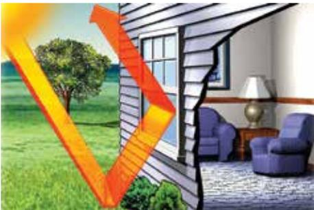
Low-E glass filters long-wave radiation from the sun. This reduces solar heat gain from the sun in the summer... keeping your home cooler.
